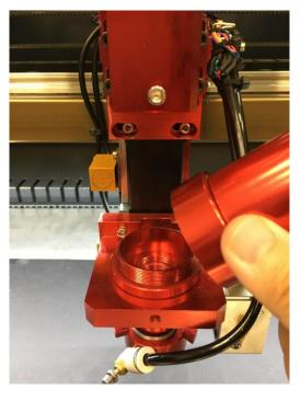
As shown below, loosen the retaining nut that is holding the Non-Metal lens housing and remove it from the laser head assembly. You'll need to unhook the 6mm hosing from the nozzle to complete
