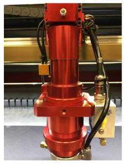
Technically, you can still use the Metal head to cut Non-Metal material. The main drawback from this is that you do NOT have the Auto-Focus Function available now that the Metal head equipped!
