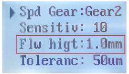
After making the changes, Press the **Enter button**, then the **Back button**. You be prompted to save the new settings. Press the **Enter button for YES** or the **Back button for NO**.
