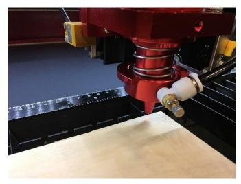
Next, go to More > Other on the Touch Panel to have the menu show up that's illustrated on the picture. If you need to bring the worktable up closer to the nozzle before Autofocusing, use the U-Axis Up/Down Arrow Keys from the main interface.
