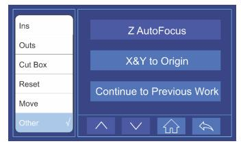
Once you have activated the Z AutoFocus, the worktable will bring the material upwards towards the nozzle of the laser head. The Z Limit Flange will then start to get closer to the proximity switch for the Z-Axis. Once the flange reaches the switch, it will then bounce the worktable back downward at the set Focal Depth.
