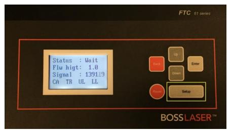
Now move the laser head's nozzle by using the Up and Down buttons from the FTC 61 Series Control Panel very close to the material, but not touching (about 5mm gap), as illustrated in the picture showing the metal head w/ the metal sheet.
