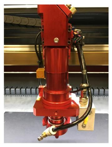
Now before we move into cutting metal with the Metal head, we need to change out the Non-Metal Lens housing & nozzle assembly to the Metal lens housing & nozzle assembly.
