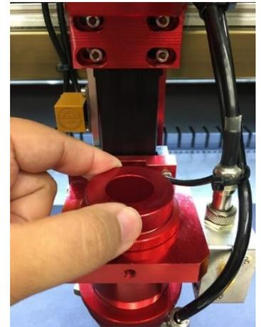
After the lens housing is secure, take the dust cover and place it over the lens housing, the edge of the dust cover should sit on the retaining nut. Once the dust cover is in place, bring the top portion of the dust cover up and tighten the set screw to secure the dust cover.
