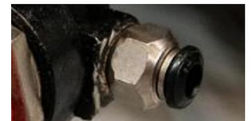
After you have changed the fitting, remove the 6mm nylon tubing from the toolbox and plug it into the air compressor fitting we just installed. Once that is complete, take the other end of the 6mm nylon tubing and plug it into the "Air In" port located on the back side of the machine.
