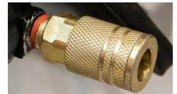
Now, take the 6mm air compressor fitting located in your toolbox and attach it to the same port that you remove the gold quick disconnect from. You may need to wrap Teflon tape around the threads of the air compressor fitting prior to screwing it into the air compressor. Use your adjustable wrench to ensure the fitting is secure and snug, be careful not to overtighten.
