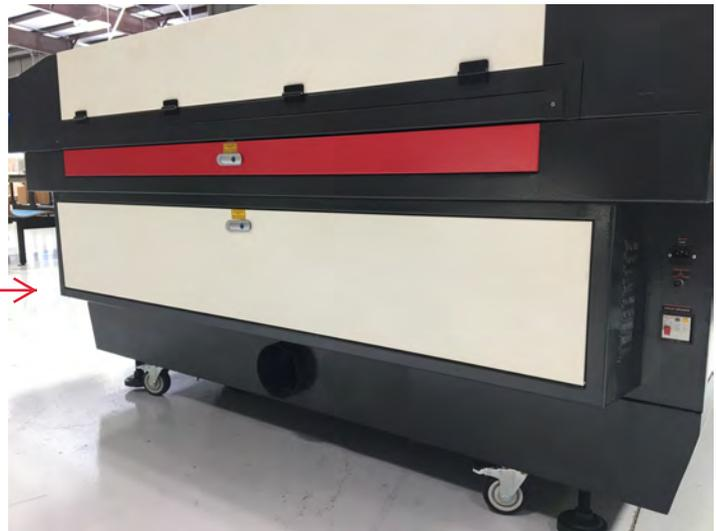
**Exhaust Port located at the bottom (ex. LS-3655 shown)**
