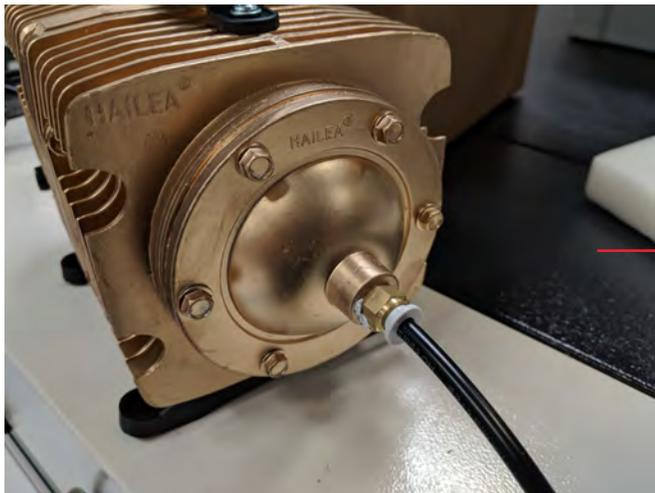
**Fitting installed w/ 6mm hosing**
