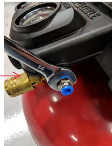
**Installing 6mm fitting using a 14mm wrench**
