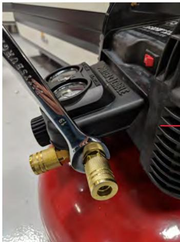
**Removing original fitting for 6mm fitting using a 19mm wrench**
