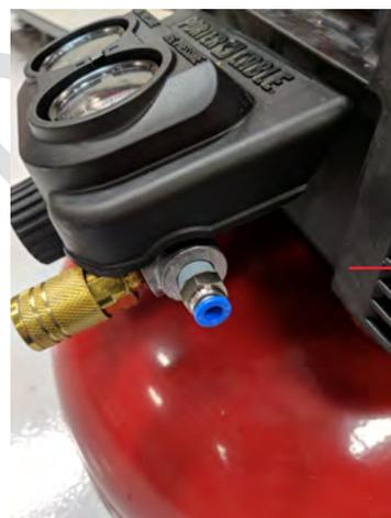
**Installed 6mm fitting onto compressor**
