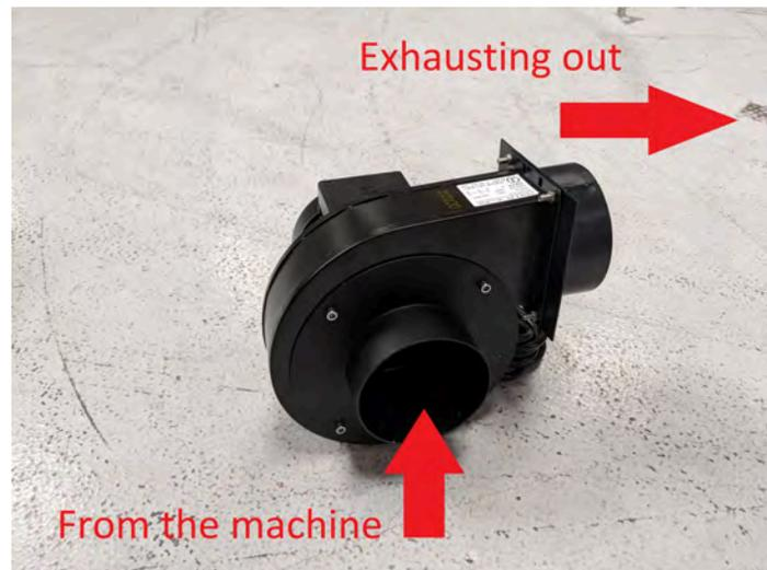
**Connect exhaust tubing from machine to intake. Then connect exhaust tubing to the exhaust port to your preference.**
