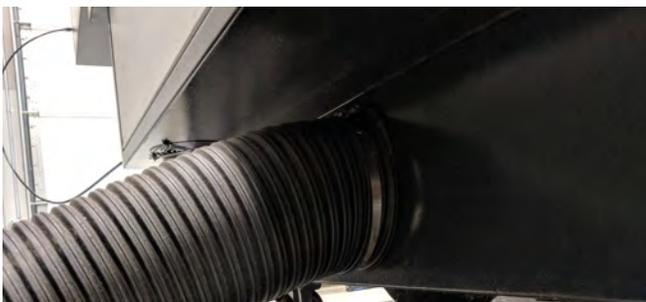
**6" Exhaust tubing installed w/ hose clamp**
