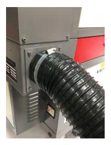
4" Exhaust Tubing Installed w/ hose clamp
