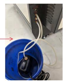
Using the 2nd silicone tubing, connect it from <u>Water Out</u> to 5 gallon bucket
