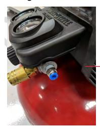
Installed 6mm fitting onto compressor
