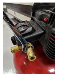
Removing original fitting for 6mm fitting using a 19mm wrench
