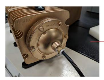
Fitting installed w/ 6mm hosing
