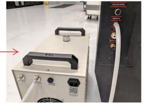
Outlet from the water chiller to Water In of the machine
