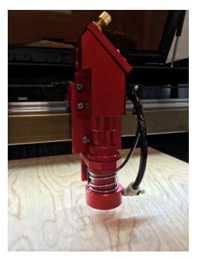
Using the 2" Focal Guide to double-check the Auto-Focus feature.
