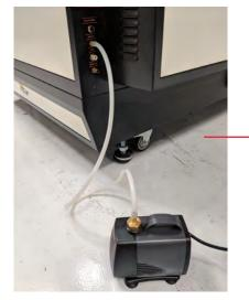
Installing silicone tubing from water pump to Water In machine
