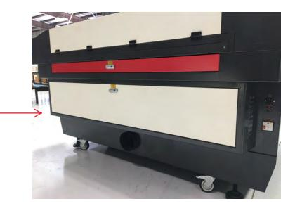
Exhaust Port located at the bottom (ex. LS-3655 shown)
