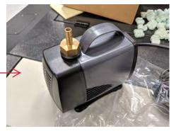
Installing fitting for silicone tubing
