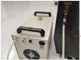
Inlet from the water chiller to Water Out of the machine
