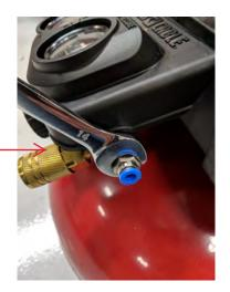
Installing 6mm fitting using a 14mm wrench
