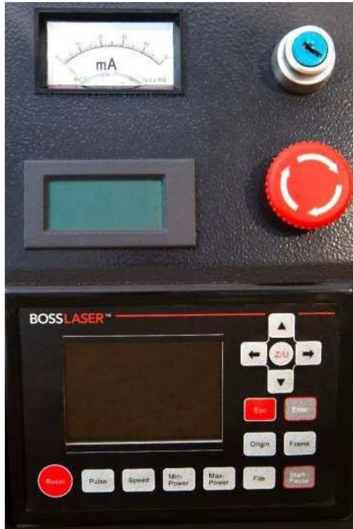
*Figure 6 LED Panel, Emergency Stop Button, Key On/Off Switch*
