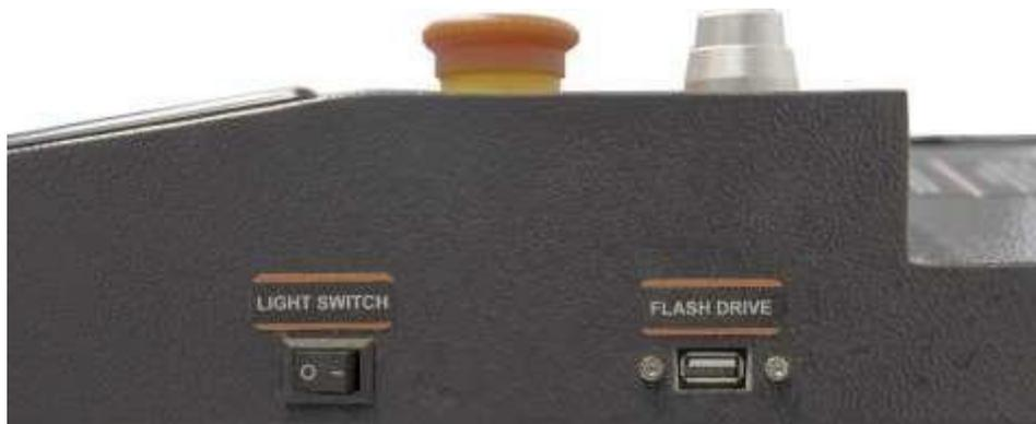
*Figure 5b USB Port and Light Switch*
