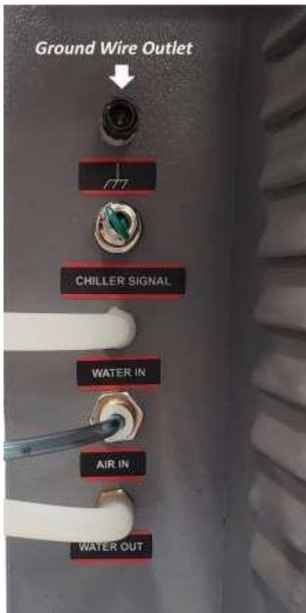
*Figure 3e Chiller Signal Outlet & Ground Wire Outlet*
