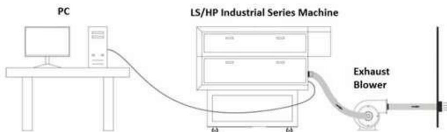
Figure 2a. Exhaust system configuration with an exhaust blower.
