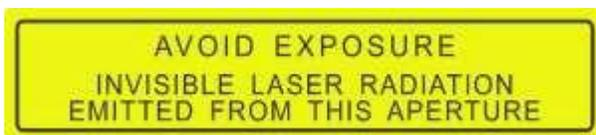
The “AVOID EXPOSURE” warning label can be found inside of the working area, on the back left-hand side behind the gantry. The aperture next to this warning label is where your laser beam will bounce from mirror #1 to mirror #2. It is important to remember that the laser beam is invisible and can cause serious injury.
